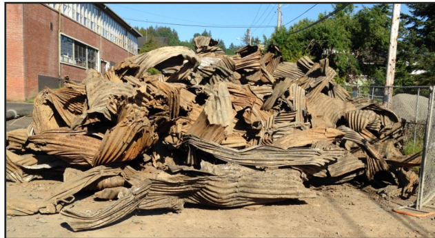
Above: Damaged and mangled pipe removed from Fox Creek. The culvert was drastically undersized for the flow levels it experienced.
