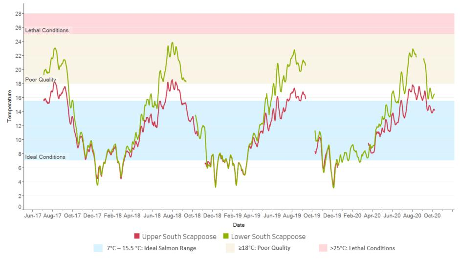
Figure 54: 7-day average maximum temperatures (7dMAM) for Upper South Scappoose and Lower South Scappoose creeks from June 2017 to October 2020 overlayed on salmonid temperature threshold ranges. See Table 3 for temperature threshold details.
