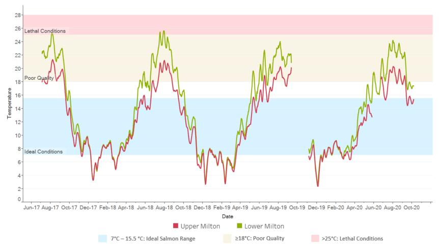
*Figure 29: Milton Creek Watershed 7-day average maximum temperatures (7dMAM) from June 2017 to October 2020, overlayed on salmonid temperature threshold ranges. See Table 3 for temperature threshold details.*
