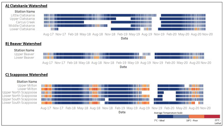
Figure 5: Data logger deployment timeline at 13 monitoring stations across three watersheds, from 2017 to 2020. The colors represent average water temperature (°C) during deployments corresponding to the temperature threshold shown in Table 3 and represented in the legend.
