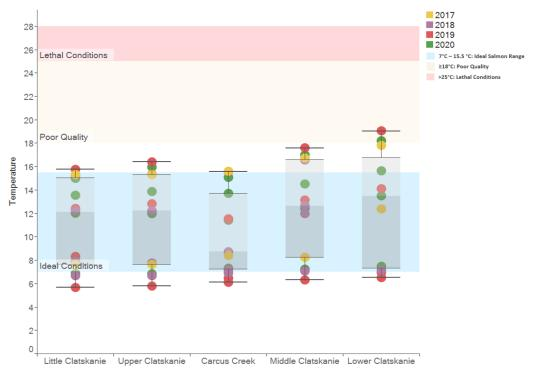
*Figure 8: Clatskanie Watershed 7dMAM Temperature range from 2017 to 2020, overlaid on the DEQ stream temperature standard ranges for healthy salmon habitat (Table 3). Data points represent the months monitored in a year.*
